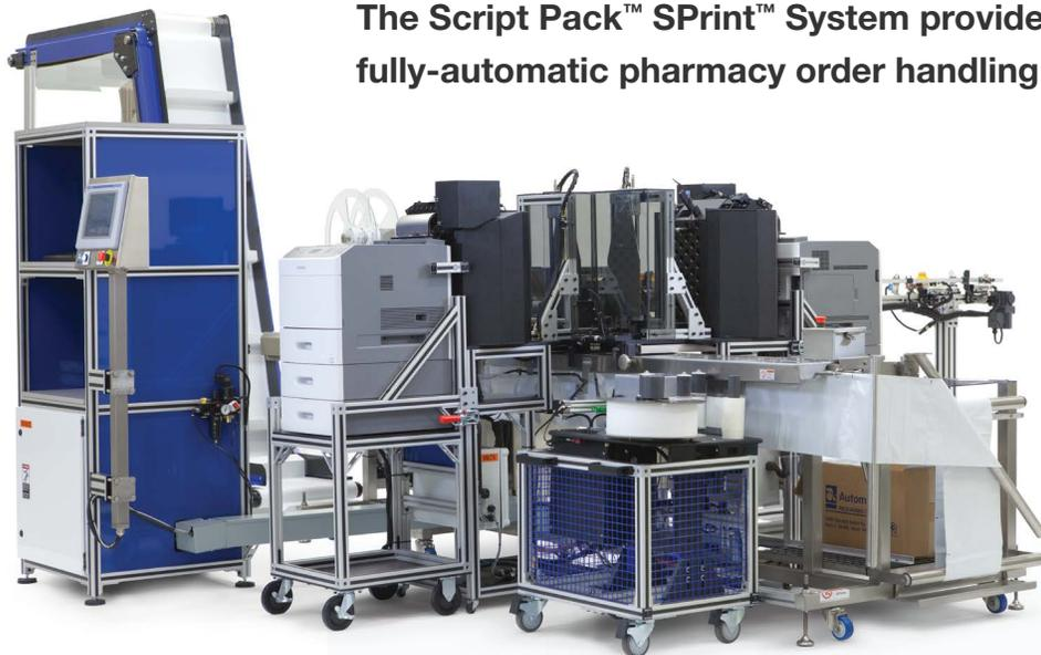
prints and indexes the Lit Packs as the orders are conveyed to the packaging station. As the verified, labeled bag is moved into loading position, the Script Pack SPrint automatically verifies, folds and inserts the correct Lit Pack for each order.
