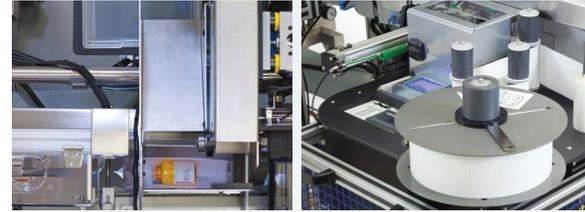
A wide bag opening enables automatic loading of single or multiple piece orders
